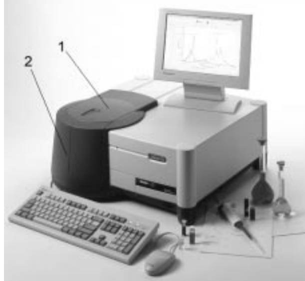
Cary Eclipse showing the sample compartment lid (1) and front panel (2)
